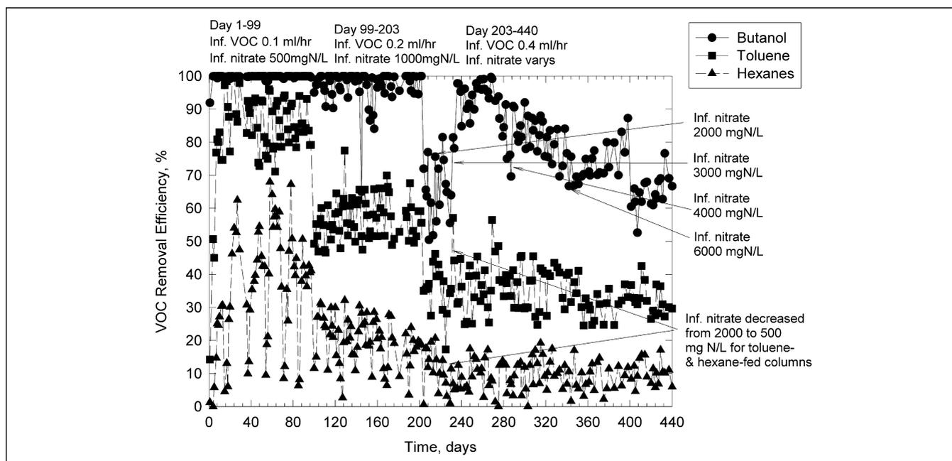
**Figure 2.** The overall biofilter performance with respect to butanol, toluene, and hexane removal.
