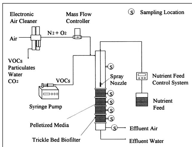
**Figure 1.** The trickle-bed biofilter system.
