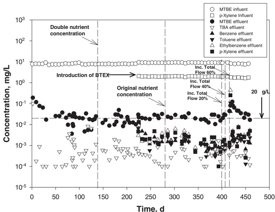
**Figure 1** Performance of fluidized bed reactor with time: influent and effluent concentrations are plotted through various stages of operation. For brevity, only p-xylene is plotted of the four influent BTEX compounds. The dashed horizontal line indicates the 20  $\mu\text{g/L}$  effluent concentration level
