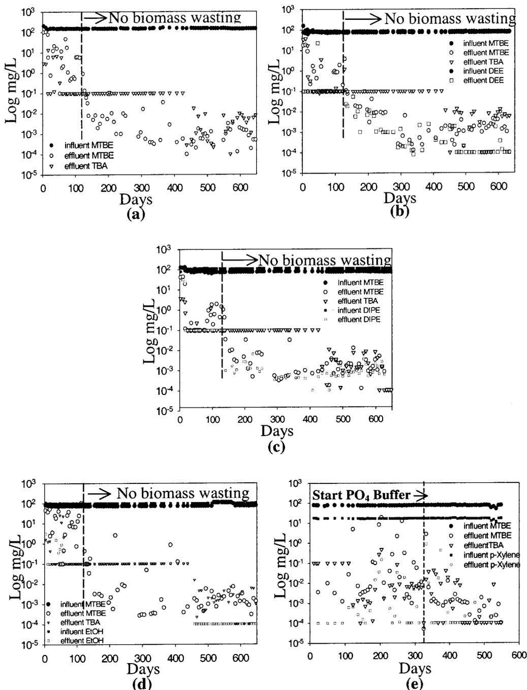
FIGURE 1. Porous-pot chemostat performance plots for (a) MTBE only, (b) MTBE and diethyl ether (DEE), (c) MTBE and diisopropyl ether (DIPE), (d) MTBE and ethanol (EtOH), and (e) MTBE and benzene, toluene, ethylbenzene, and *p*-xylene (BTEX). Method detection limit of *tert*-butyl alcohol (TBA) shifted from 0.1 mg/L to 0.1  $\mu$ g/L midway through the study. For simplicity, only *p*-xylene is plotted of the four BTEX compounds
