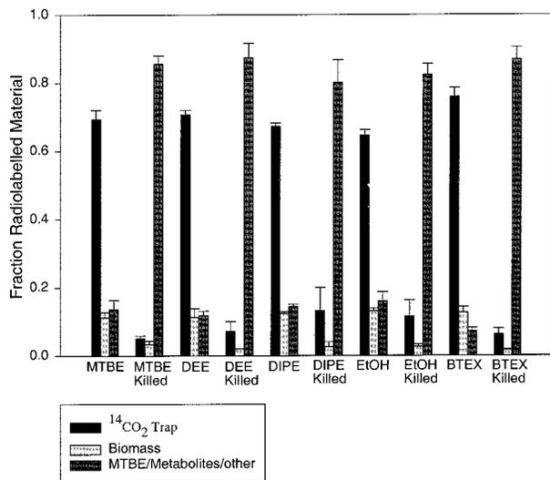
FIGURE 2. Radiolabeled <sup>14</sup>C-MTBE fate study. Size of bar indicates fraction of radioactivity found in each of three regions: 0.5 M KOH<sup>14</sup>-CO<sub>2</sub> trap, biomass, and the filtrate containing any remaining <sup>14</sup>C-MTBE or intermediates. Error bars indicate standard deviation of quadruplicate samples.
