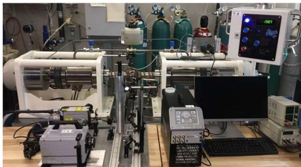
Figure 1. Photograph of the RCM setup
