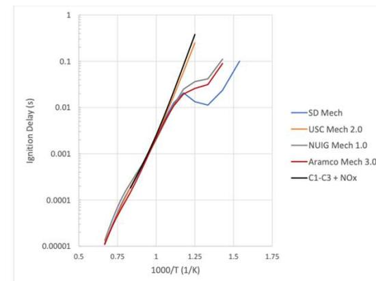
Figure 2. Demonstrated differences in mechanisms running at 30 bar
