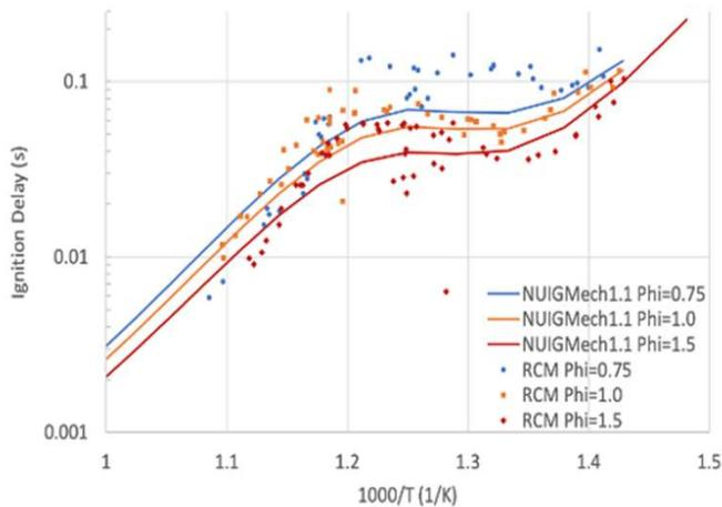
**Figure 3.** Experimental ignition delay measurements and simulated delays of propane / oxygen / inert mixtures at 24 bar with NUIGMech1.1 mechanism
