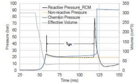
**Figure 4.** Experimental vs. simulation pressure data with volume of chamber
