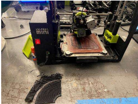
Fig 12. Delamination on \frac{1}{4} of the disk
