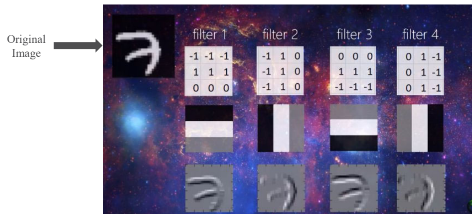
Figure 1. Shows an example of a Neural Network Running Network trained to look for edges – the white parts of each photo show the top, bottom, left, and right edges of the original photo
