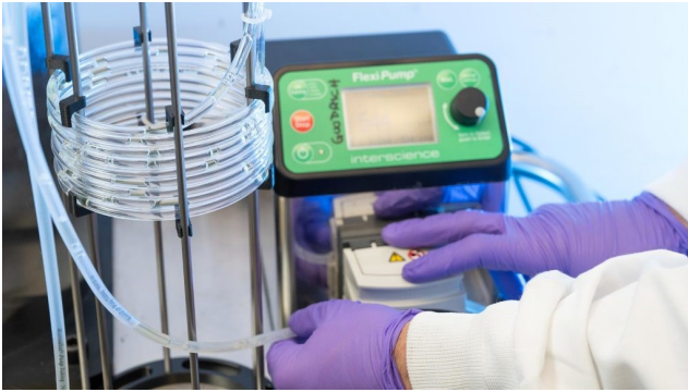
The VacciRAPTOR's custom engineering includes a coil system through which the virus solution flows while being exposed to UV light.
