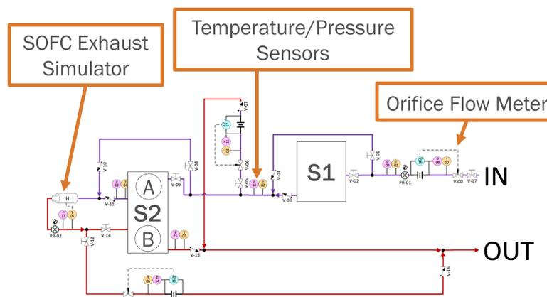
Figure 5: Test bench piping and instrumentation diagram.
