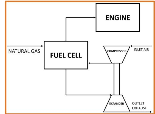
Figure 1: Simplified hybrid SOFC/IC schematic (adapted from [1]).
