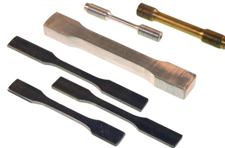
“Dog-bone” shaped samples for tensile test
