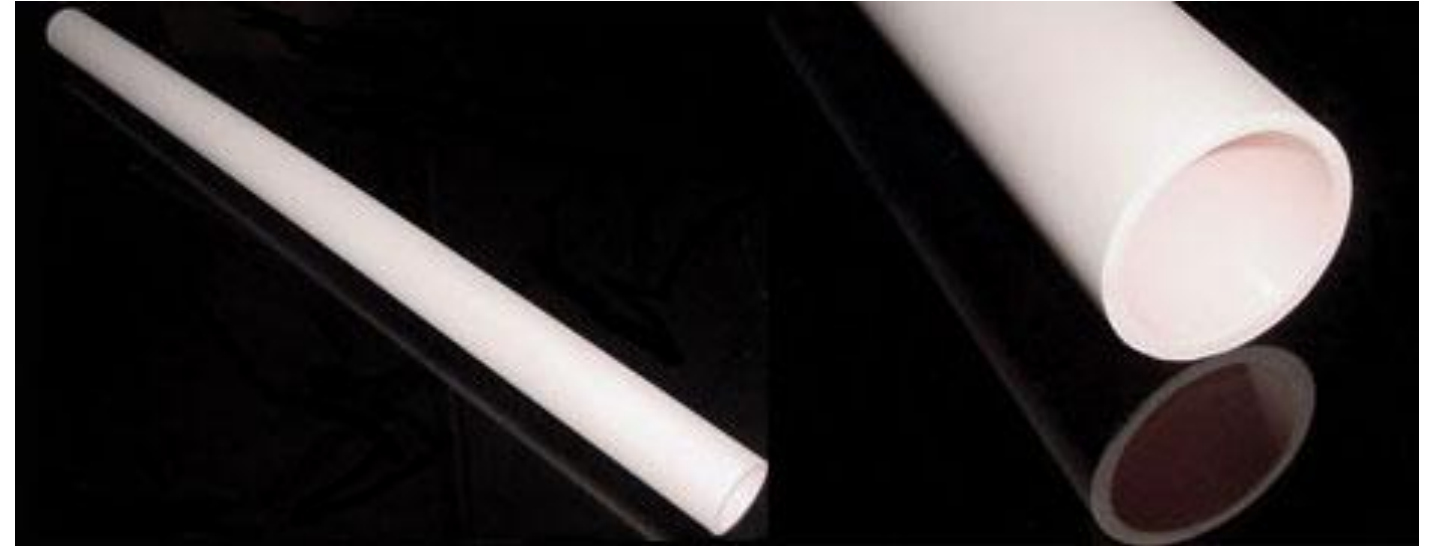
Al 2 O 3 tube for tube furnace, melting point: T m = 2025°C
