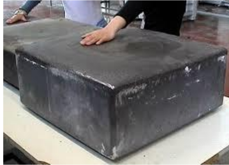
Casted poly-crystalline Si
