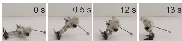
Fig. 11. Experimental results for transition from wheeling mode to jumping mode.
