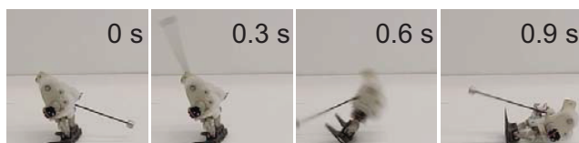
Fig. 12. Experimental results for transition from jumping mode to wheeling mode.
