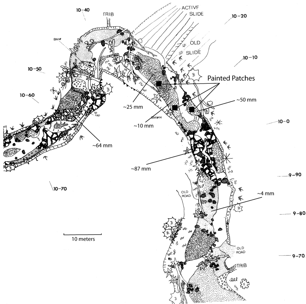
Figure 1. Facies map of Wildcat Creek, near Berkeley, CA, showing locations used in the painted rock study. Numbers along border are distances in meters. Tree locations along the bank are indicated by various symbols. Large woody debris is shown roughly to scale. Average median grain sizes are indicated for each facies type, and area with no pattern was covered by water. Flow is from left to right.
