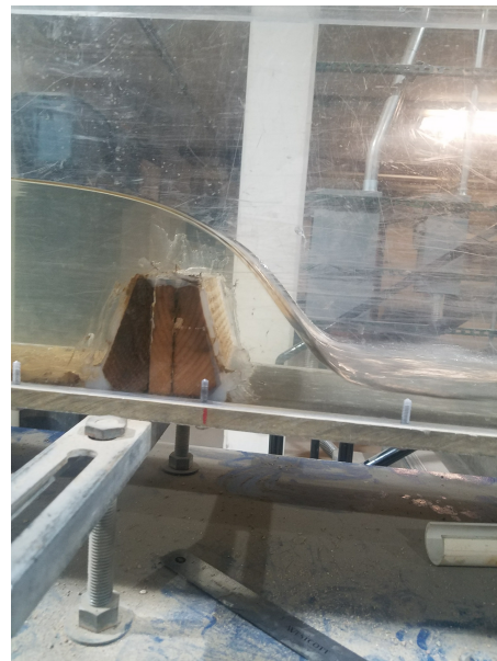
Figure 2.1: View of flume experiment with dam in the middle of the flume
