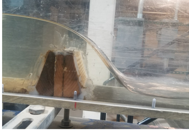
Figure 3.1: View of the experimental set up in the flume with the dam and the curvilinear flow over the dam in the case of where the discharge is 0.16 cfs (Run B.1).
