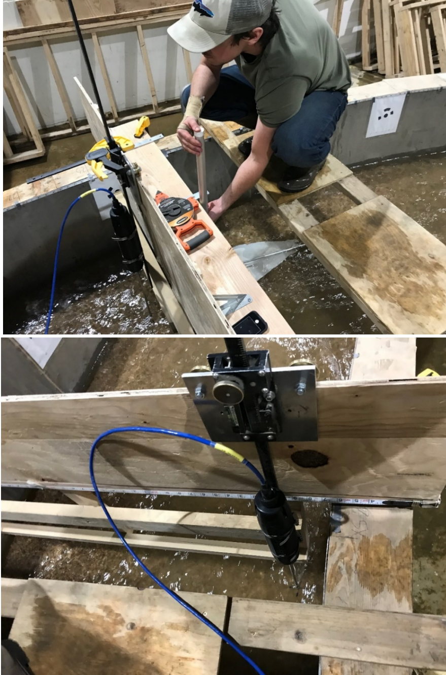
Figure A1. We used a Helley-Smith bed load sampler and sampled over periods ranging from 45 to 120 seconds. The bottom picture shows our velocity measurement configuration using a Vectrino ADV which we mounted to a rolling track.
