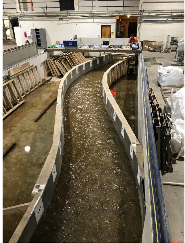
Figure A2. These two pictures show the flume set up with water being pumped and sediment fed into the channel. The picture on the left is looking upstream and the figure on the right is looking downstream.
