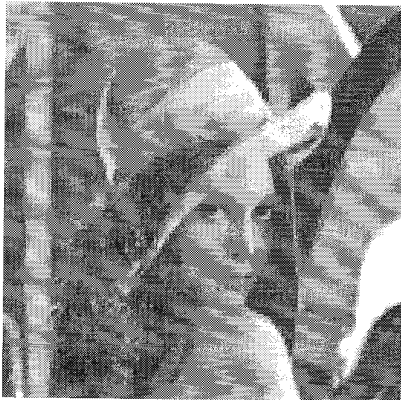
Fig. 5. Reconstructed image using RLS for 16 \times 16 lattice. (SNR = 35.7 dB).
