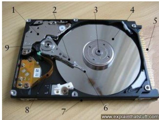
To read data, hard drives make use of a part called a head, labeled #6 in the diagram above. The head is basically a piece of metal that's wrapped in wire. When a reading data from the disk the arm, #2 above, will move the head to a specific location on the disk while the disk is spinning at several thousand revolutions per minute (RPM). What happens in the head component which allows the rest of the computer to process the data (hint: it processes the data as an electrical signal)?
