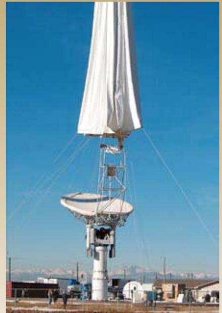
*New antenna technology, which was installed last spring, improves the CHILL radar’s dual-polarization capabilities. Many TV stations nationwide will upgrade to dual-polarization systems.*
