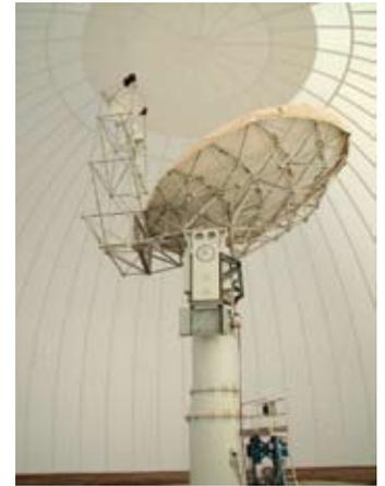
*This spring, new antenna technology was installed on the CHILL radar. When looking straight up, the highest point of the antenna is approximately 50 feet above the ground. The antenna is made of aluminum and weighs nearly 6,000 pounds.*
