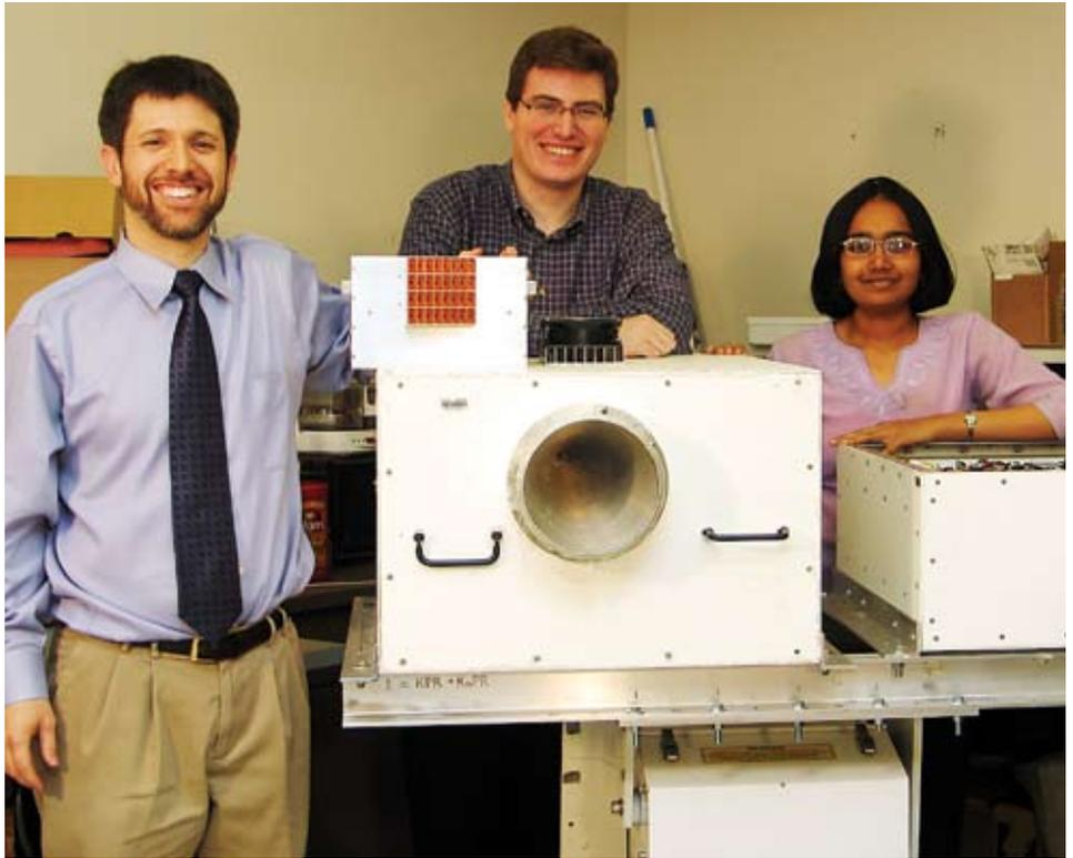
*Dr. Steven Reising, left, and his graduate students have been performing extensive research in miniaturizing passive microwave instruments for ground-based use. The instrument (pictured on top) was built with significantly reduced mass, volume, and power consumption relative to conventional radiometers (bottom instrument). The team is working with Ball Aerospace & Technologies Corp. to adapt what they already have learned to a space-based environment.*
