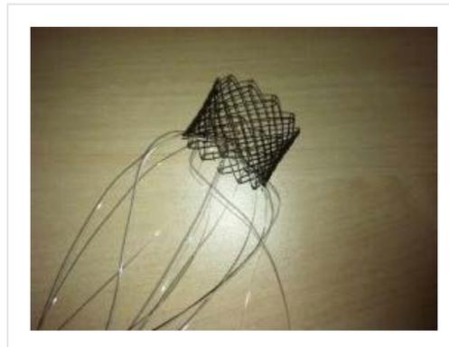
The team created the new valve out of nitinol, a flexible nickel titanium shape memory alloy. To move it, doctors would lace six threads through the stent using a special rod and pull it into place. The valve collapses under the pressure of being pulled and then regains its shape.
