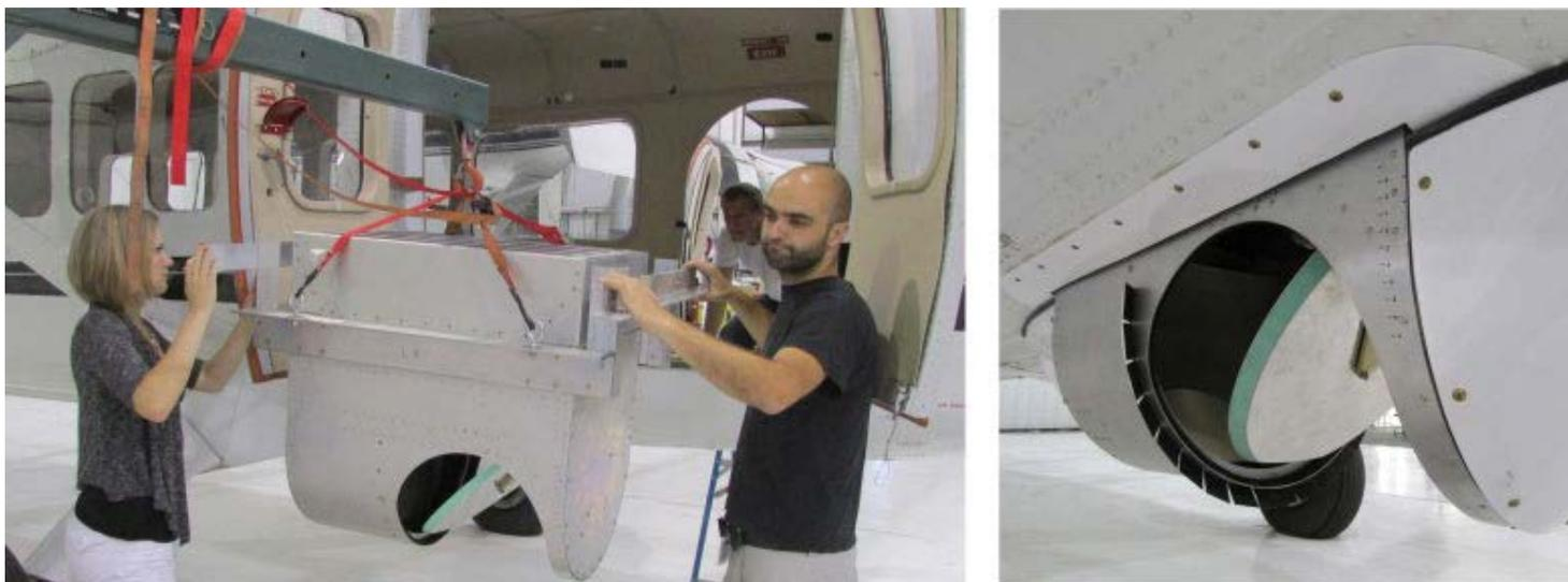
*Above left: HAMMR team members Torie Hadel and Xavier Bosch-Lluis install the instrument into the Twin Otter. Right: The fairing with the microwave reflector for scanning across the scene. (Images: S. Reising, Colorado State Univ.)*
