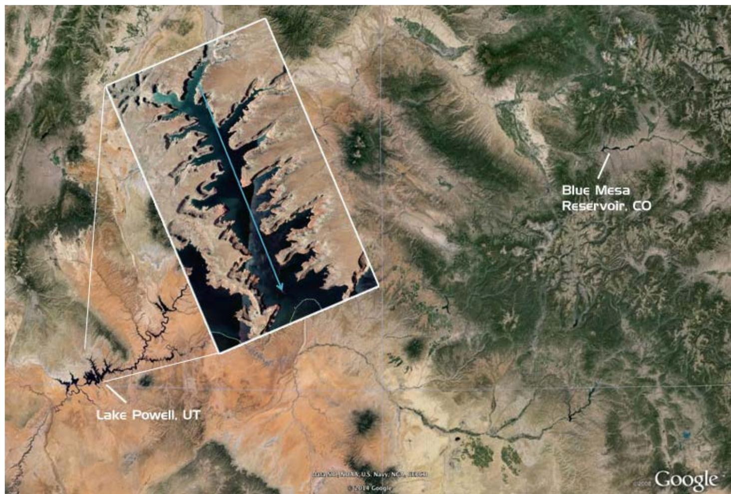
*On Wednesday, July 9, HAMMR had a two-hour instrument checkout flight over Blue Mesa Reservoir in Colorado. On July 10th and 11th, HAMMR made more extensive engineering flights totaling approximately 12 hours over Lake Powell in Utah. Lake Powell was chosen as a large inland body of water with a number of clear land-to-water transitions. The inset map shows one of the flight lines over Lake Powell. (Image credit: Google Earth)*
