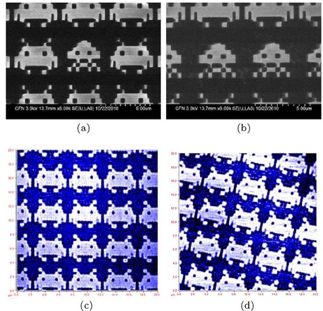
Fig. 3. (Color online) Electron microscope scans of the two Talbot masks used in the experiment with on-purpose fabricated defects. (a) Defect equivalent to a single unit cell. (b) Defect equivalent to an entire row of cells. (c) Corresponding AFM scans of the reconstruction at first Talbot plane corresponding to a mask with a single cell defect. (d) A mask with entire row of defects.
