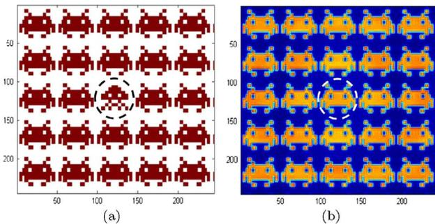
Fig. 2. (Color online) Numerical simulation of the defect-tolerance concept of the GTI for a mask composed of 10,000 cells. (a) Mask with a defect. (b) Intensity distribution at the Talbot plane. The reconstruction does not show the defect indicated in the dashed lined circle.
