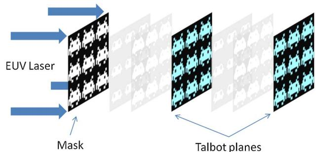
Fig. 1. (Color online) Experimental setup. The EUV laser illuminates the Talbot mask that renders self-images at the Talbot planes where the sample is located.
