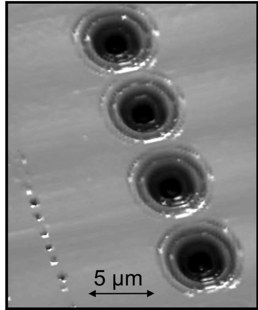
Fig. 3. AFM image of ablation craters produced by EUV laser ablation in PMMA using the unattenuated beam with first diffraction-order focusing (far right, unoptimized sample position) and third diffraction-order focusing (center and left).
