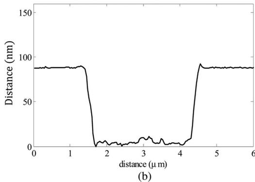
Fig. 5. Trenches machined on PMMA with a 46.9-nm laser beam positioning the sample at three different distances from the third-order focus of the zone plate and attenuating the beam by  $\sim 8\times$ . (a) Cross-section of the groove on the left along its length. The groove a has a FWHM of 160 nm and a width at the surface of 250 nm. (b).
