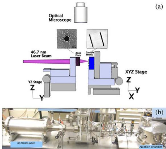
Fig. 1. (a) Schematic representation of the setup used to demonstrate EUV laser nanomachining. The output of a 46.9-nm capillary discharge EUV laser is focused with a FZP lens onto the sample. (b) Photograph of the nanomachining laser system showing the 46.9-nm capillary discharge laser (left) is attached to the processing chamber (right).
