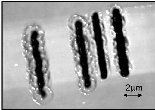
Fig. 4. Trenches machined on PMMA with the unattenuated 46.9-nm laser beam by positioning the sample at four different distances near the first-order focal plane. The left-most trench has an average width of  $1\ \mu\text{m}$ , and the diameter of the surrounding rings approach  $2\ \mu\text{m}$ .
