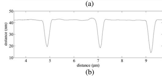
Fig. 6. Trenches machined on PMMA with a 46.9-nm laser beam by positioning the sample at three different distances from the third-order focus of the zone plate attenuating the beam by  $\sim 16\times$ . The groove on the left has an FWHM of 130 nm and a width at the surface of 200 nm.
