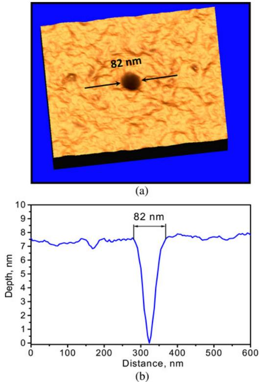
Fig. 2. AFM image (top) and lineout (bottom) of a 82-nm diameter hole ablated on PMMA by a single shot from a 46.9-nm laser. The sample was placed at  $7\ \mu\text{m}$  from the third-order focal plane of the one plate (from [10]).
