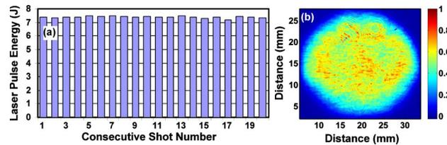
Fig. 2. (Color online) (a) Shot-to-shot variation of amplified  $\lambda = 800$  nm Ti:sapphire laser pulse energy measured at a 1 Hz repetition rate. The average laser pulse energy is 7.4 J, and the standard deviation  $\sigma = 1\%$ . (b) Typical intensity profile of the amplified  $\lambda = 800$  nm beam.
