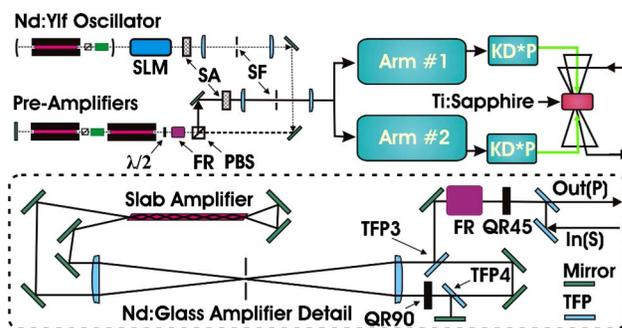
Fig. 1. (Color online) Top, block diagram of the third amplification stage of the Ti:sapphire pump laser system and associated slab amplifier laser system. Bottom, schematic diagram of the eight-pass Nd:glass slab amplifier.
