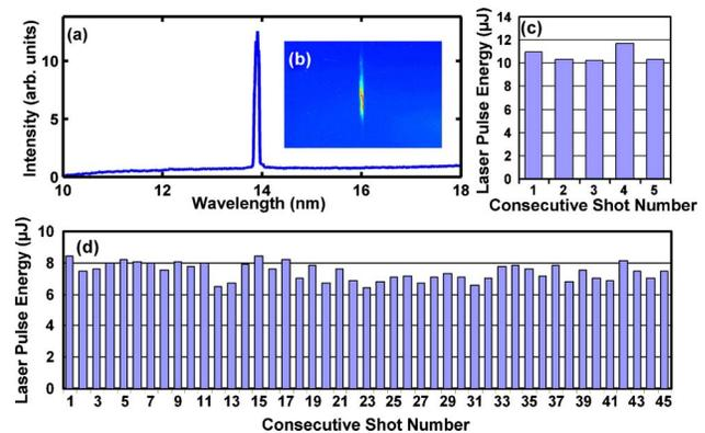
Fig. 3. (Color online) (a) Spectra of the Ni-like Ag plasma amplifier, showing highly monochromatic laser emission at  $\lambda = 13.9$  nm. (b) Spectrally resolved CCD image of the laser output. (c) Laser output pulse energy of the  $\lambda = 13.9$  nm laser operating at 0.5 Hz and (d) 2.5 Hz SXR laser operation with an average energy of  $7.4 \mu\text{J}$  with a shot-to-shot laser pulse energy variation of  $\sigma = 7\%$ .
