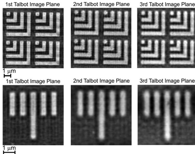
FIG. 5. AFM images of 500 nm test patterns recorded at several Talbot planes in 50 nm thick PMMA.
