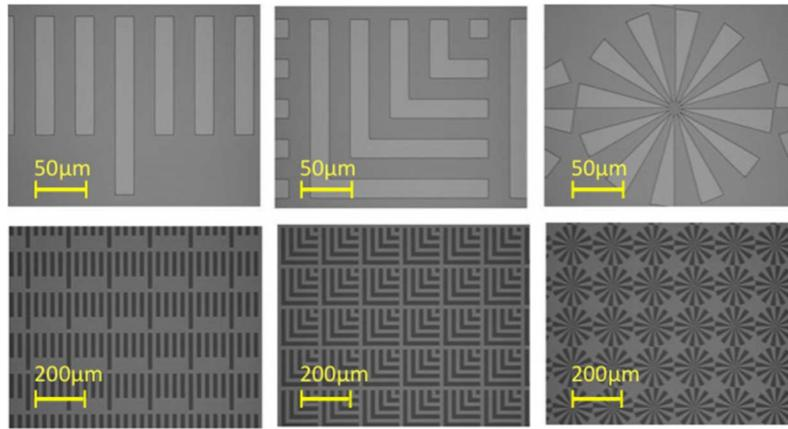
FIG. 3. (Color online) Optical microscope images of the GTI mask.
