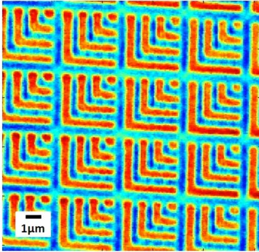
FIG. 7. (Color online) AFM scan of Talbot imaging on the sixth plane. The sixth Talbot distance is  $\approx 6$  mm, and the pattern is still imaged faithfully.
