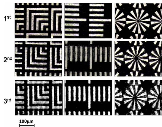
FIG. 4. (Color online) Digital charge-coupled device (CCD) camera recorded images of Talbot imaging at first (10.24 cm), second (20.48 cm), and third (30.72 cm) Talbot planes using He–Ne laser light. Notice the ringing due to the highly coherent imaging conditions.
