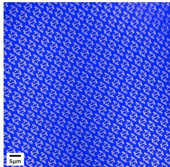
FIG. 6. (Color online) AFM images of 140 nm test patterns rotated by  $45^\circ$  recorded at the first EUV Talbot plane in 50 nm thick PMMA.
