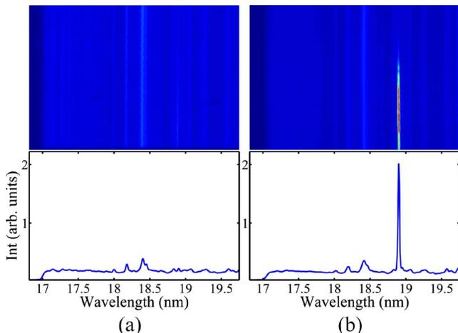
Fig. 4. (Color online) (a) On-axis soft x-ray spectrum taken with a total pump energy on target of 0.7 J. (b) The same spectrum taken with 0.94 J of pump energy, showing lasing in the 18.9 nm laser line of Ni-like Mo.
