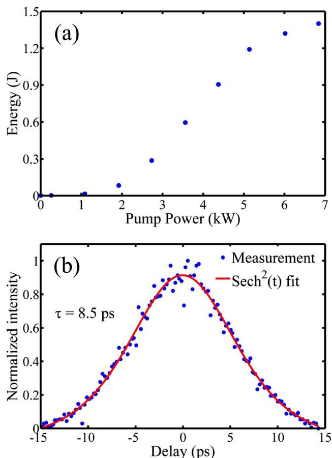
Fig. 3. (Color online) (a) Uncompressed Yb:YAG laser output pulse energy as a function of pump peak power from 2 ms pump pulses. A maximum energy of 1.45 J was obtained with a peak pump power of 7 kW. (b) Hyperbolic secant square fit of the autocorrelation data corresponding to 8.5 ps FWHM pulses.
