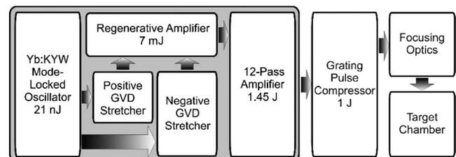
Fig. 1. Block diagram of the diode-pumped soft x-ray laser. The oscillator, stretchers, and amplifiers are shown to fit on a single 12 ft  $\times$  5 ft optical table.
