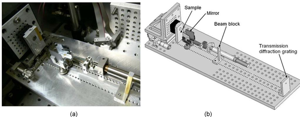
**Fig. 6** Amplitude division interferometric lithography setup. The laser beam is split using a transmission diffraction grating into two beams corresponding to the two first diffraction orders. The two beams are recombined in the sample surface on reflections in two grazing mirrors.
