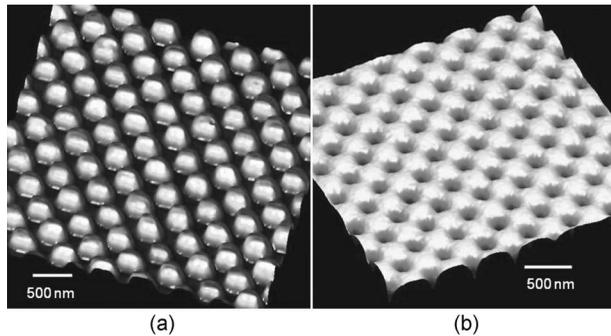
**Fig. 5** (a) Dots and (b) holes fabricated in HSQ with a Lloyd's mirror interferometer and two successive exposures. The change from dots to holes is obtained by changing the exposure dose. The FWHM of the holes is 130 nm, and the depth is 120 nm.
