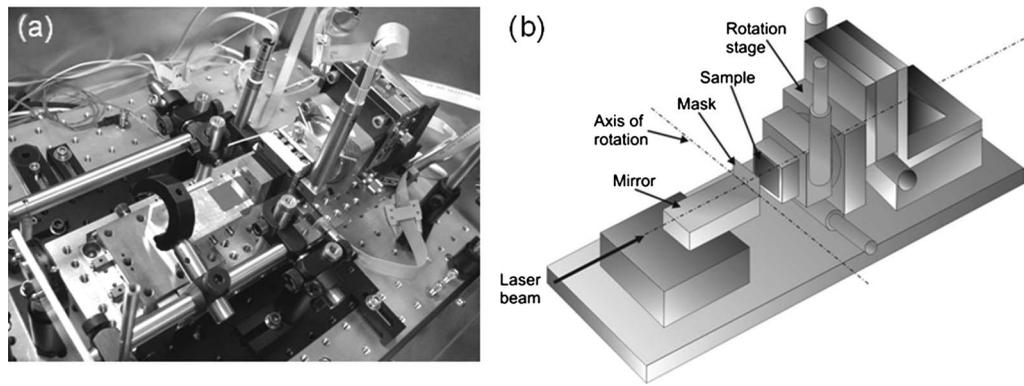
**Fig. 3** Wavefront division interferometer based on a Lloyd's mirror. The setup allows for multiple exposures of the sample with arbitrary rotation angles around an axis parallel to the mirror's surface.
