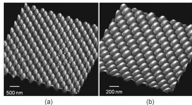
**Fig. 4** Arrays of symmetric (a) and elongated (b) nanodots printed in PMMA using a Lloyd's mirror interferometer with two successive exposures after rotating the sample by an angle  $\alpha = \pi/2$  and  $\alpha = \pi/6$ , respectively.
