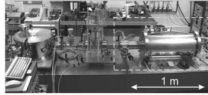
**Fig. 1** Tabletop  $\lambda = 46.9$ -nm laser and experiment chamber. The footprint of the system is  $2.5 \times 0.75$  m<sup>2</sup>.
