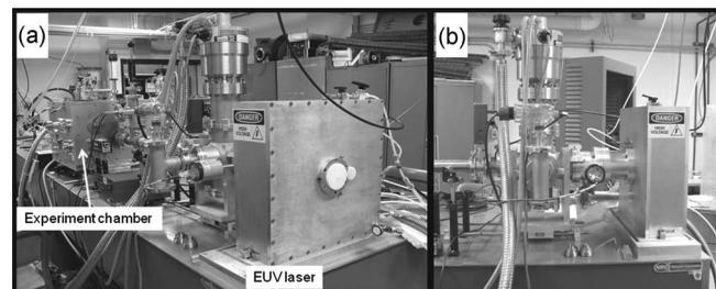
**Fig. 2** (a) Photograph of the desktop capillary discharge laser (right) connected using a vacuum manifold to the experiment chamber (left) housing the amplitude division interferometer. (b) Desktop version of the capillary discharge laser with an energy per pulse about 10  $\mu\text{J}$  and a repetition rate up to 12 Hz.
