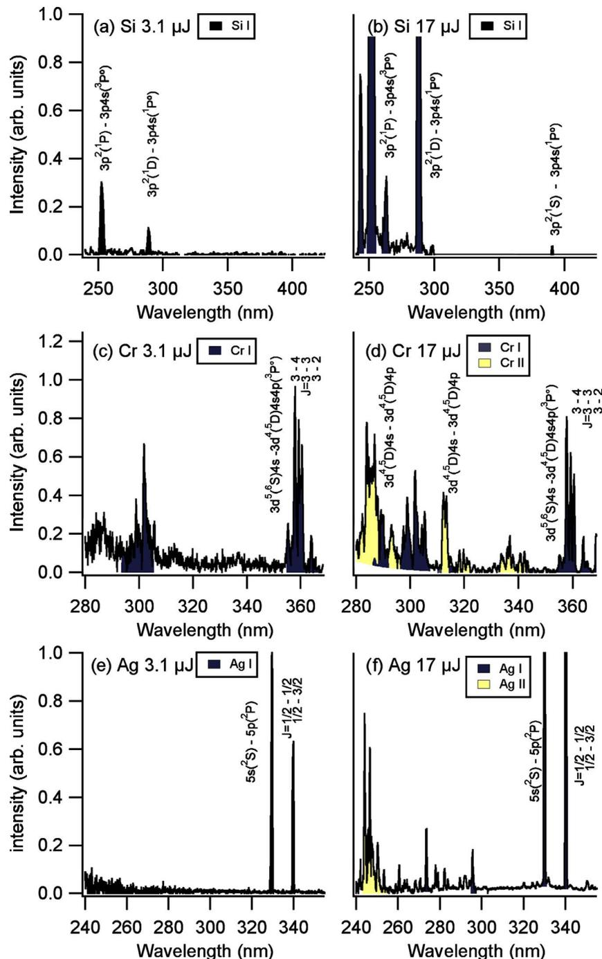
Fig. 2. (Color online) Spectra of Si, Cr, and Ag plasmas created by irradiating solid targets with 3.1 and 17  $\mu\text{J}$ , 46.9 nm soft-x-ray laser pulses. At 3.1  $\mu\text{J}$  (a) Si is only slightly above the ablation threshold, while for both (c) Cr and (e) Ag strong lines from the neutral atoms are present. At 17  $\mu\text{J}$  only neutral atom lines are present for (b) Si, while the (d) Cr and (f) Ag spectra show lines from both the neutral atoms and the singly charged ions.
