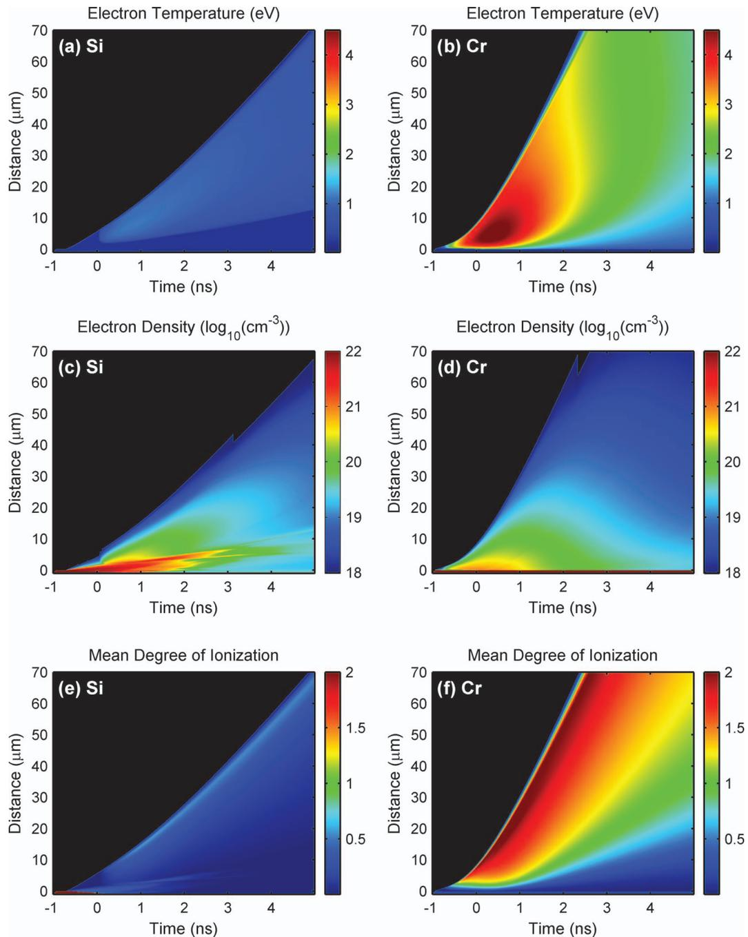
Fig. 3. Computed plasma parameters corresponding to Si and Cr plasmas generated by  $17 \mu\text{J}$  energy, 1.2 ns duration soft-x-ray laser pulse irradiation ( $\lambda=46.9 \text{ nm}$ ) of solid targets. Because of the smaller absorption cross section (a) the Si plasma is significantly colder than (b) the Cr plasma. (d) The Cr plasma expands at a significantly higher rate. Due to the lower temperature (e) the Si plasma has a much lower degree of ionization than (f) the Cr plasma.
