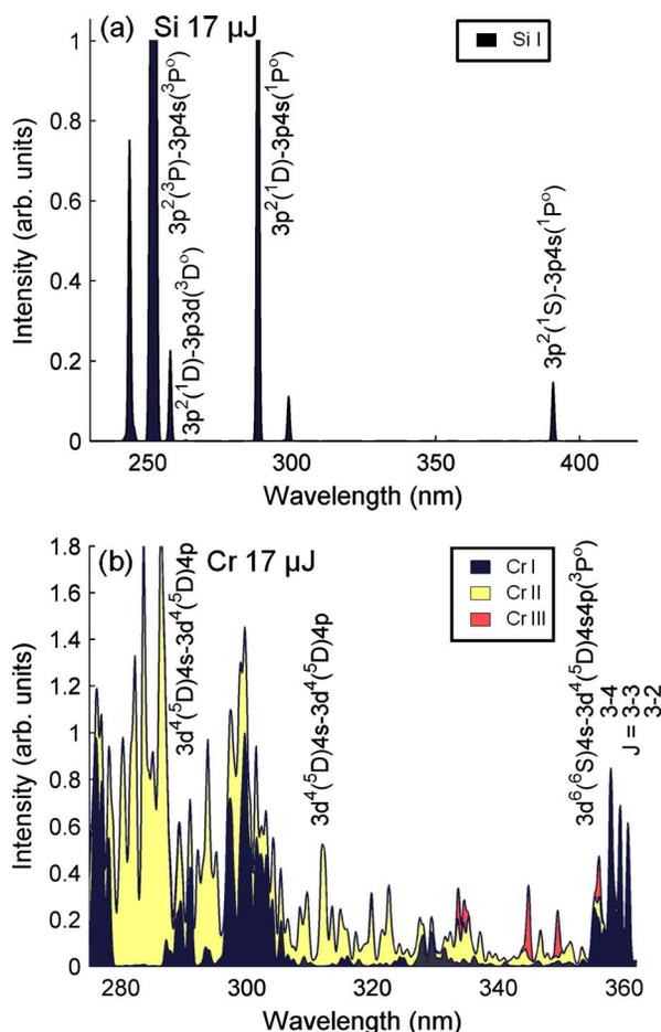
Fig. 4. (Color online) Simulated spectra for Si and Cr plasmas created by  $17\ \mu\text{J}$  soft-x-ray laser ( $\lambda=46.9\ \text{nm}$ ) pulse irradiation. (a) The Si spectrum is completely dominated by neutral atom lines (Si I) (a), while (b) the hotter Cr spectra contain large numbers of both Cr I and Cr II lines.
