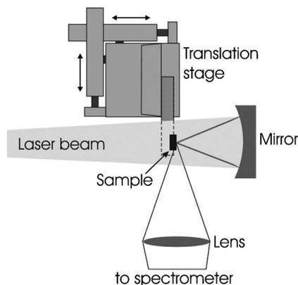
Fig. 1. Experimental setup used for the generation and spectroscopy of soft-x-ray laser-created plasma. The vacuum chamber is not shown.
