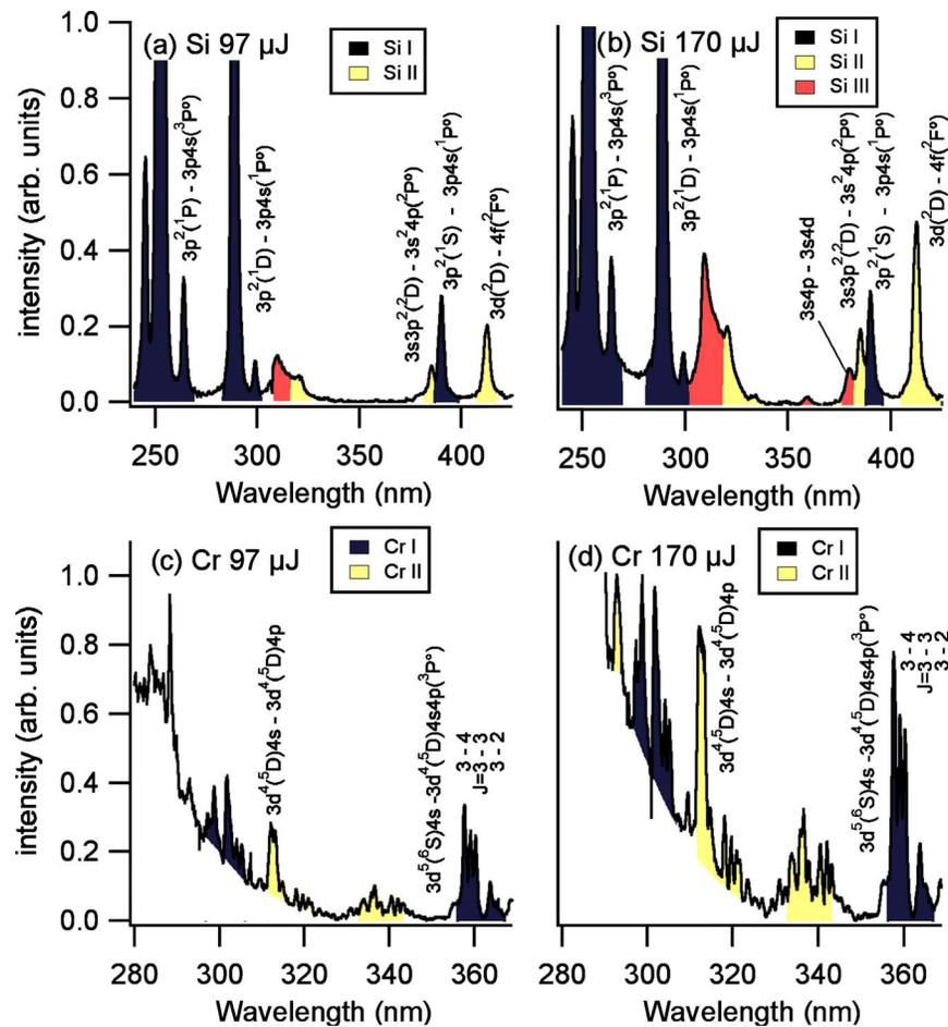
Fig. 5. (Color online) Spectra of (a), (b) Si and (c), (d) Cr created by  $\lambda=800$  nm laser pulses of 120 ps duration. Si II, Si III, and Cr II lines are emitted from the plasmas created by the 90 and 170  $\mu\text{J}$  pulses.
