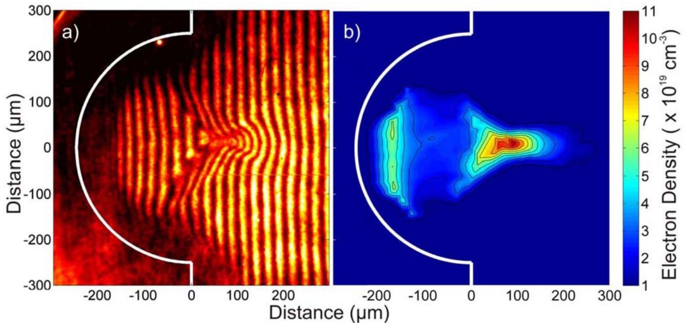
Fig. 1. (a) Soft X-ray interferogram of a plasma created by the laser irradiation of a 500- $\mu\text{m}$ -diameter semicylindrical Al cavity at an intensity of  $1.1 \times 10^{12} \text{ W} \cdot \text{cm}^{-2}$  with a 120-ps-duration laser pulse and (b) the resulting electron density map. The interferogram depicts the plasma at 4.4 ns after the peak of the laser irradiation pulse.
