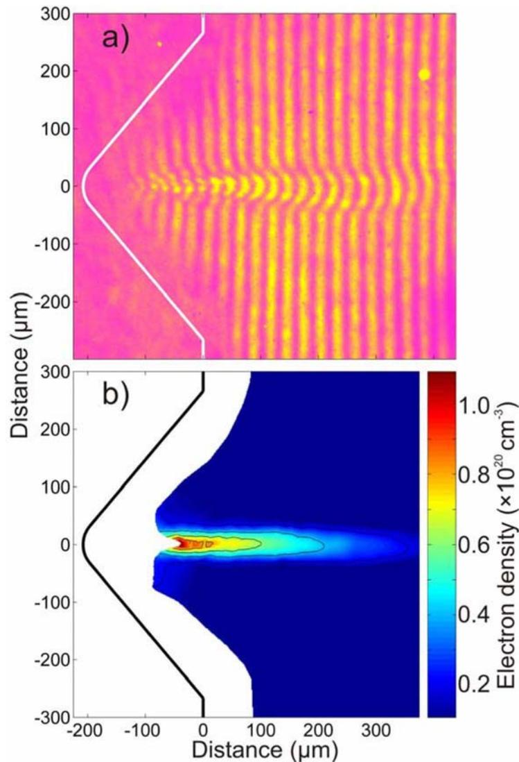
Fig. 1. (a) Soft X-ray interferogram and (b) corresponding plasma density map of a plasma jet created by the laser irradiation of a triangular copper groove. The interferogram is taken 4.2 ns after the irradiation of the target surface (outlined on the figure by the solid black line) by a 120-ps-duration optical laser pulse with an intensity of  $1.1 \times 10^{12} \text{ W} \cdot \text{cm}^{-2}$ .
