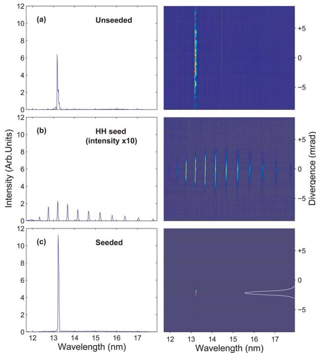
Fig. 1. (Color online) Spectra of (a) unseeded 13.2 nm Ni-like Cd laser, (b) HH seed pulse, and (c) seeded laser. The Cd plasma amplifier was pumped by a 0.85 J short pulse configured into a 3.5 mm FWHM long line focus.
