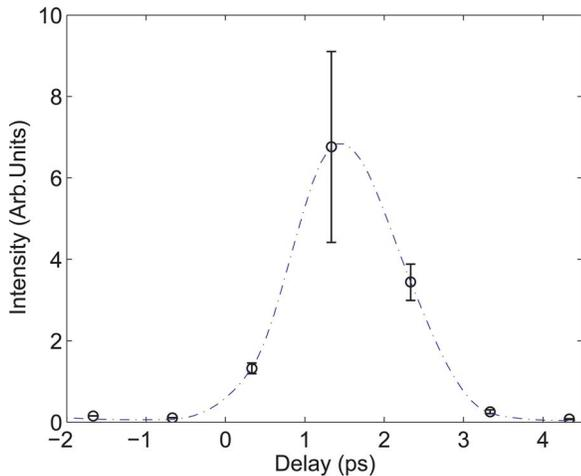
Fig. 3. Intensity of the amplified seed pulse as a function of time delay between the peaks of the short pump pulse and the seed pulse at the target position.
