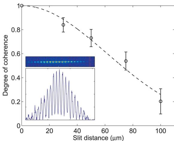
Fig. 4. (Color online) Degree of coherence  $|\mu_{12}|$  of the seeded laser beam as a function of slit separation. The slits were placed at 10 cm from the exit of the amplifier. The inset shows a single shot interferogram and corresponding lineout for the 30  $\mu\text{m}$  slit pair.
