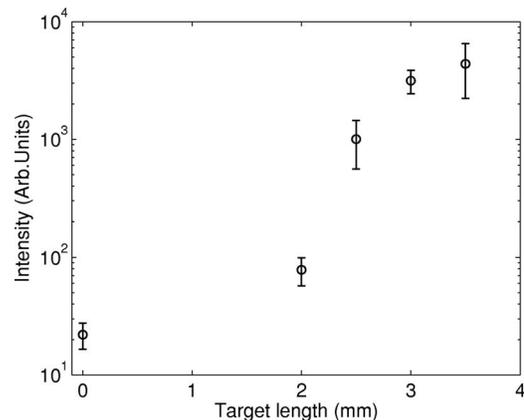
Fig. 2. Variation of the intensity of the 13.2 nm amplified seed pulse as a function of the Ni-like Cd amplifier plasma column length.
