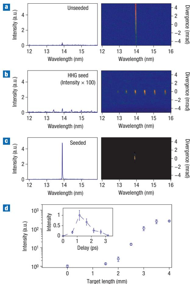
**Figure 3** Characterization of seeded 13.9-nm nickel-like silver laser.
