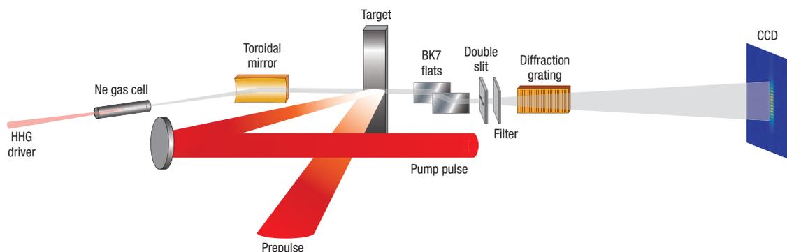
**Figure 1** Schematic diagram of the injection-seeded, nickel-like SXL. The main optical laser pulse exciting the amplifier impinges at  $23^\circ$  grazing incidence onto the target. A neon gas cell is used to generate the high harmonic seed. The set-up used to measure the spatial coherence is shown to the right of the amplifier. HHG stands for high harmonic generation.
