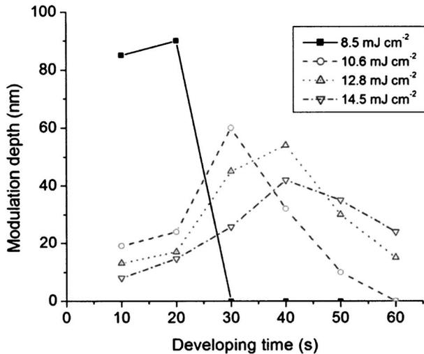
FIG. 3. Modulation depth for an array of holes with  $\sim 500$  nm period as a function of the developing time for different doses.
