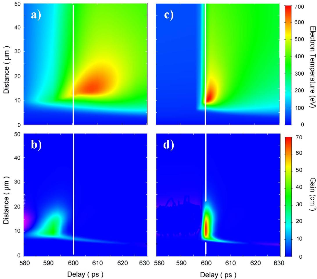
FIG. 5. (Color online) Calculated spatiotemporal distribution of the temperature and gain in Ni-like Mo for pump pulse durations of 12 ps [left pictures (a) and (b), respectively] and 2 ps [right pictures (c) and (d), respectively]. The delay between the 120 ps prepulse and the pump pulse is 600 ps. The vertical white line shows the time of the peak intensity of the pump pulse.
