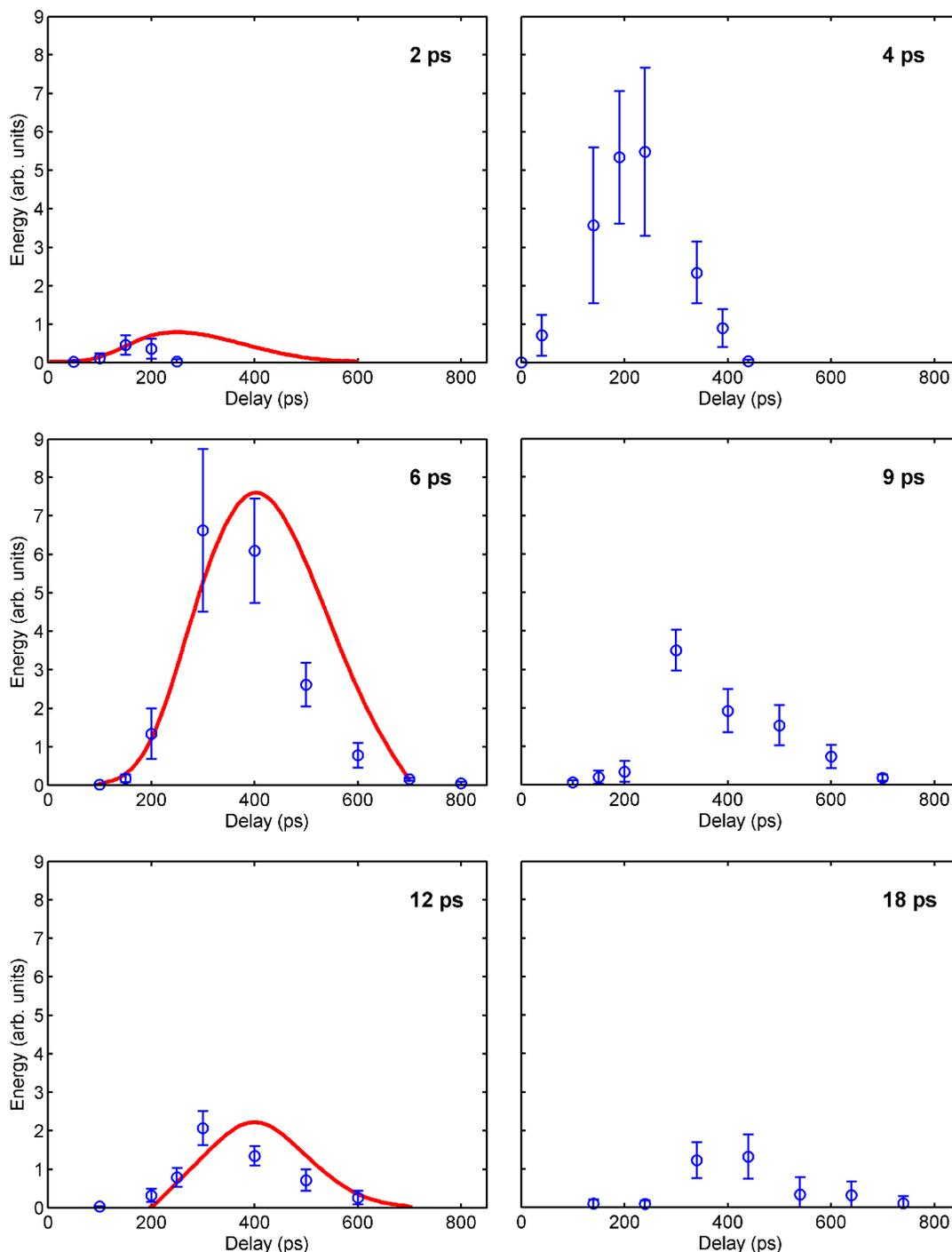
FIG. 2. (Color online) Measured (circles) and simulated (line) laser output pulse energy variation for the 13.9 nm Ni-like Ag laser as a function of time delay between the prepulse and pump pulse for pump pulse durations between 2 ps and 18 ps. Each point in the graphs is an average of about ten laser shots. The energy of the short pump pulse was 1 J.
