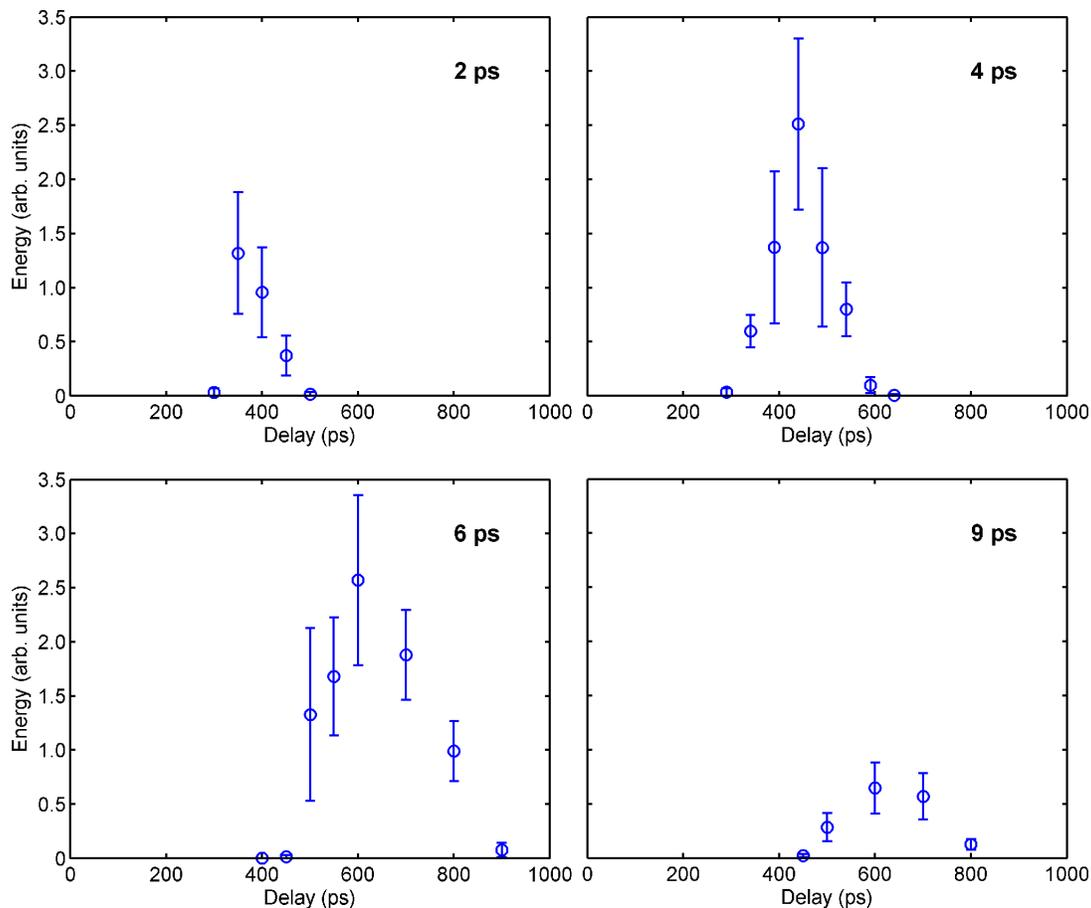
FIG. 3. (Color online) Measured laser output pulse energy variation of the 32.6 nm Ne-like Ti laser as a function of time delay between the pre-pulse and pump pulse for pump pulse durations between 2 ps and 9 ps. The energy of the peak intensity of the pump pulse was 1 J.
