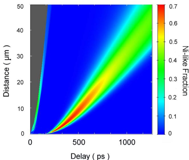
FIG. 4. (Color online) Computed relative abundance of Ni-like Mo as a function of distance to the target and time as calculated by the code. Maximum abundance in color scale is 70% and includes the region from the target surface at 200 ps to 10  $\mu\text{m}$  from the target at 500 ps. For an accurate color map please see the online version.
