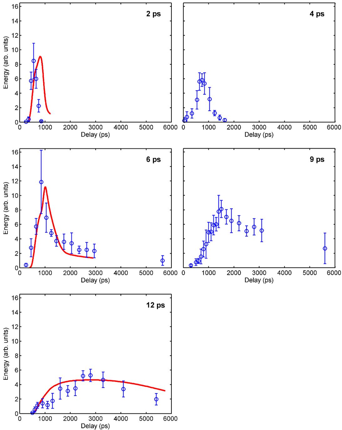
FIG. 1. (Color online) Measured (circles) and simulated (line) laser output pulse energy variation for the 18.9 nm Ni-like Mo laser as a function of time delay between the prepulse and pump pulse for pump pulse durations between 2 ps and 12 ps. Each point in the graphs is an average of about ten laser shots. The energy of the short pump pulse was 1 J.
