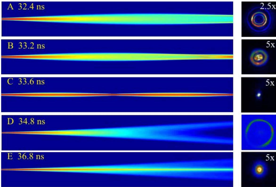
Figure 2. Modeled cross sections showing the calculated guided beam propagation in a 5.5 cm capillary (left), and corresponding experimental exit mode images (right, with magnification given).
