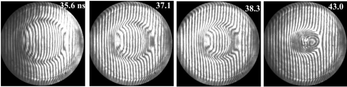
Figure 1. Time progression of interferograms showing the plasma column compression and waveguide development for a 250 mTorr Ar discharge in a 3.2mm diameter, 11cm long capillary. Times are measured with respect to the current pulse.
