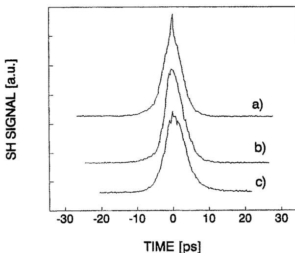
FIG. 2. Autocorrelation signal of the orange (a) and the red (b) pulses obtained by second harmonic generation (SHG) in LiIO<sub>3</sub> 1 mm thick. Pulse widths are calculated to be 5 ps assuming hyperbolic secant squared pulse profiles. Cross-correlation signal (c) obtained by sum frequency generation in KDP using a pump and probe setup, obtained without lock-in techniques.
