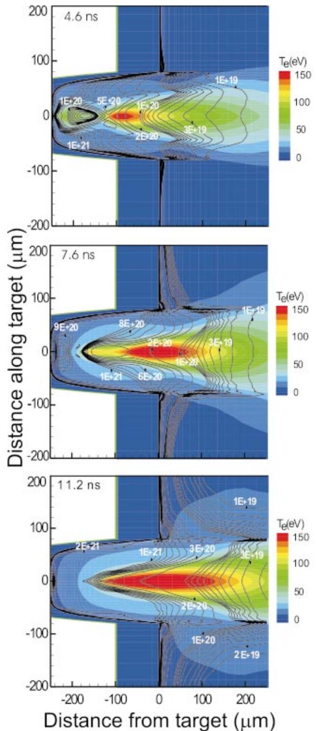
FIG. 8. (Color) Sequence of simulated electron density (line contours) and temperature (filled contour) profiles for the spot-focus plasma of Fig. 7 computed using LASNEX. The  $1 \omega$  of heating laser is incident from the right.
