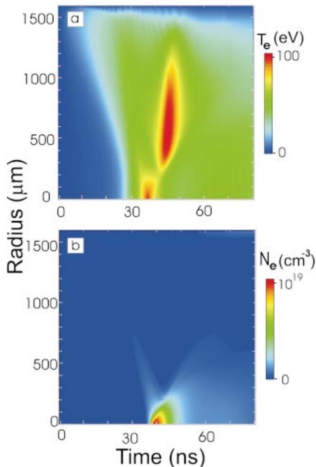
FIG. 1. (Color) Simulated spatio-temporal distribution of the (a) electron temperature and (b) electron density in a capillary discharge argon plasma column. The calculation is for an alumina capillary 3.2 mm diameter filled with 460 mTorr of Ar excited by a current pulse with a peak amplitude of 25 kA and 30 ns rise time.
