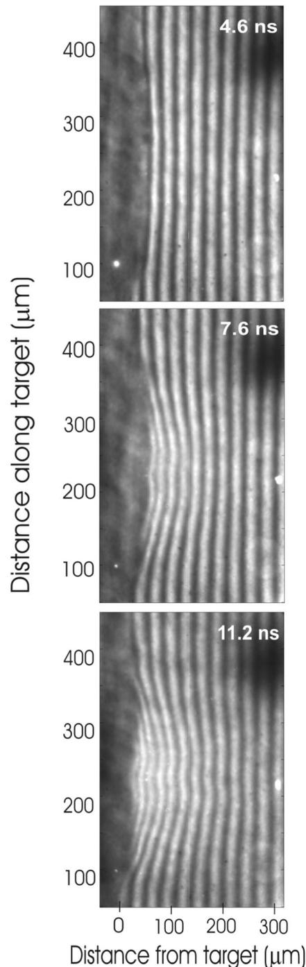
FIG. 6. Sequence of interferograms corresponding to spot-focus plasmas generated by firing a fifth shot in the same target location. The spot diameter was  $\sim 30 \mu\text{m}$  and the beam intensity was  $7 \times 10^{12} \text{ cm}^{-3}$ . The times indicated are measured with respect to the beginning of the laser pulse.
