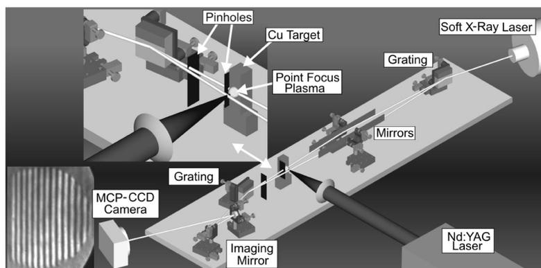
FIG. 3. A schematic representation of the amplitude division soft x-ray laser interferometer based on diffraction gratings. The interferometer was positioned  $\sim 2$  m from the exit of the soft x-ray laser. The detector was placed  $\sim 7$  m from the interferometer. An interferogram obtained with no plasma present is shown.
