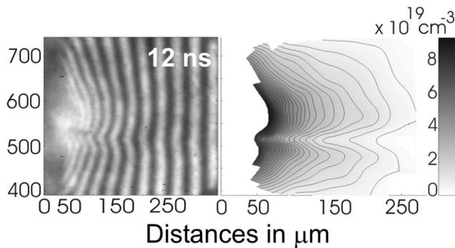
FIG. 4. An on-axis interferogram of line-focus plasma generated by irradiation of a copper target with an intensity of  $\sim 1 \times 10^{11} \text{ W cm}^{-2}$  (left), and corresponding electron density profile (right). The width of the line focus was  $30 \mu\text{m}$ .
