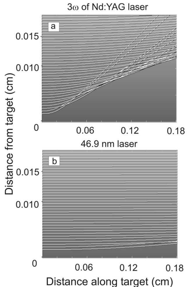
FIG. 5. Computed ray trajectories of a probe beam propagating along the axis of a line-focus plasma corresponding to the interferogram of Fig. 4 for (a) third harmonic of Nd:YAG laser, (b) 46.9 nm soft x-ray laser.
