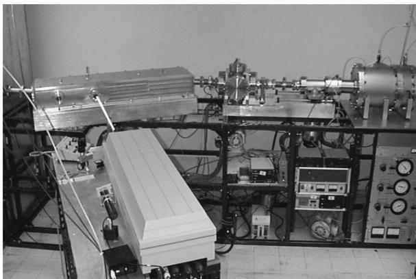
FIG. 2. Setup for soft x-ray laser plasma interferometry experiments. The capillary discharge soft x-ray laser observed on the right of the photograph generates a 46.9 nm wavelength beam that propagates into the amplitude division soft x-ray interferometer seen at the left. A commercial 1 J Nd:YAG laser used to generate the laser-created plasmas studied is seen in the lower part of the figure.
