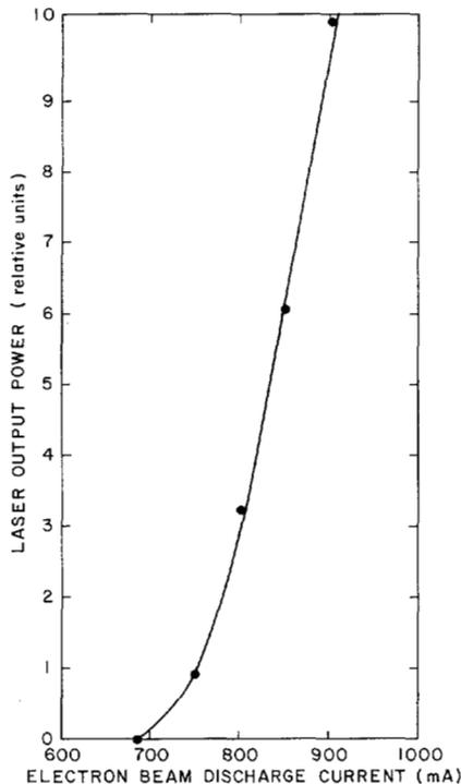
Fig. 3. Variation of the laser output power of the 6511.7 Å line of As II as a function of electron beam discharge current. The As reservoir temperature was 387°C and the magnetic field was 4 kG. The helium average pressure in the plasma tube was 1.3 torr. The electron beam energy at 900 mA was 2.7 keV.
