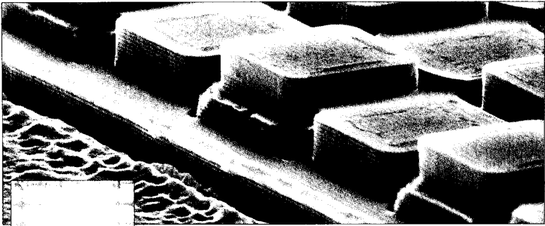
In this scanning electron micrograph, the "checkerboard" is actually a two-dimensional phased-locked array of vertical-cavity surface-emitting lasers. Molecular beam epitaxy was employed to grow the semiconductor wafer, complete with mirrors [light and dark stripes], and the result was topped by a thick phase-shift layer [solid light layer]. Then reactive ion beam etching was used to define each laser individually as a square, measuring 5 \mu\text{m} on a side, and the thick phase-shift layer was etched off the top of every other laser in the array. The inset is an optical micrograph of light emitted from the operating array.
