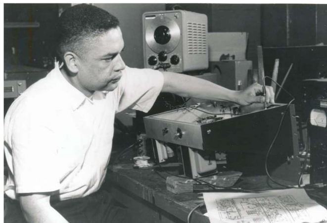
Fig. 10. Hubbard in 1951 working on electronic circuitry for the hot-wire anemometer used in water flow. (Image courtesy of IIHR.)
