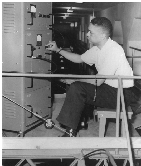
Fig. 13. Hubbard with the control box for the hot-film anemometer used in IIHR's towing tank, 1956. (Image courtesy of IIHR.)
