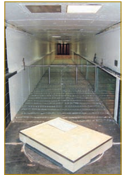
Representative wind tunnel configuration for testing of models of photovoltaic roofing systems, at the Wind Engineering and Fluids Laboratory, Colorado State University.
