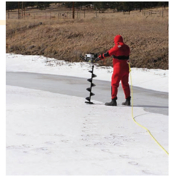
A member of the Four Mile fire district in Teller County operates an automatic auger to assist a senior design team in their survey of an erosion control dam. He is wearing a gummy suit for protection in case of a fall through the ice.
