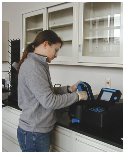
Liz Fagen measures the concentration of total phosphorus in a water sample from the Big Thompson River using a Hach DR-4000 spectrophotometer donated by Hach Chemical Company in Loveland, Colorado.
