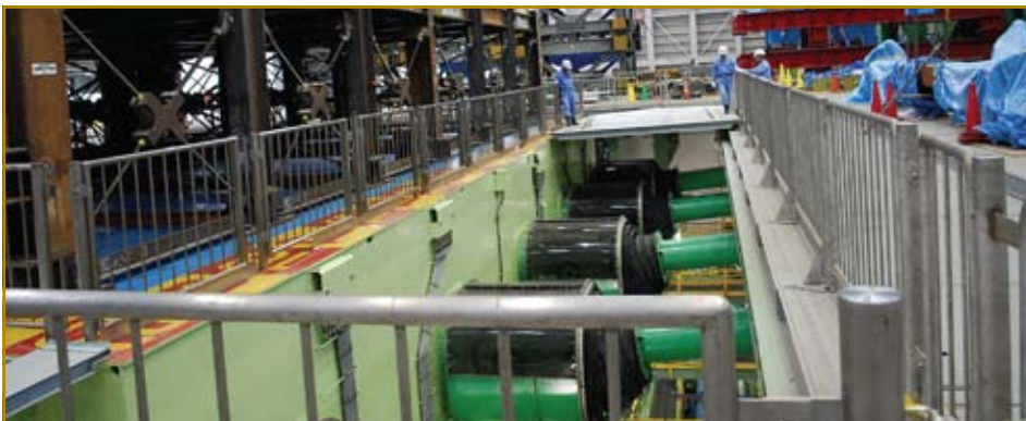
Actuators exposed the day before testing. The shake table is triaxial, meaning it can move in all three directions simultaneously.
