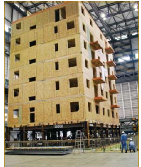
The capstone building on the shake table, ready for testing.
