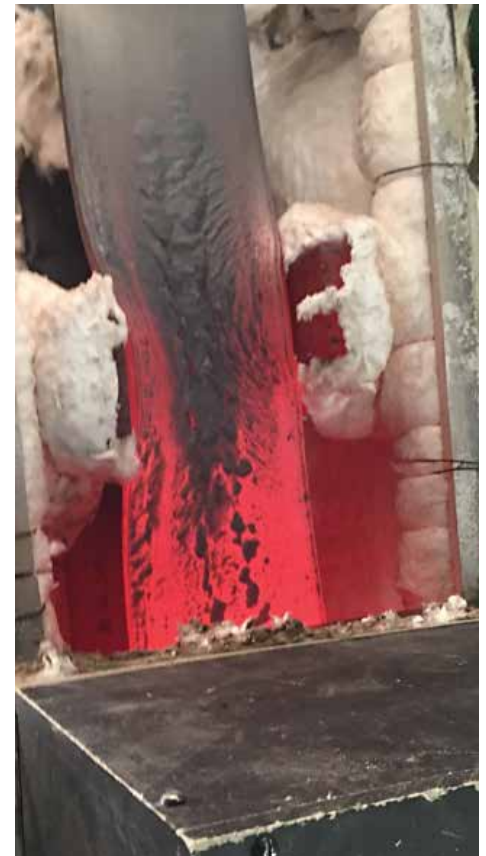
Fig. 1. Tested beam under fire
