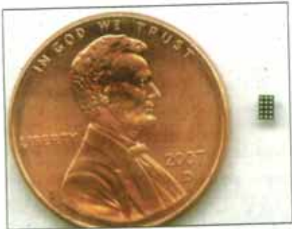
Fig. 2. Chip-scale packaging has enabled the miniaturization of linear battery-charger circuits.
