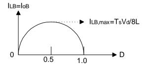
For fixed V<sub>o</sub>;  $(I_{vo})_{max}$  for a buck converter occurs at D = 0. But D=0 means V<sub>d</sub> =V<sub>in</sub>= infinite ,via  $I_{LB}(max) = I_0/D$
