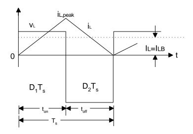
The average output current,  $I_{LB}$ (average),also occurs at CCM-DCM boundary. We choose to examine the case  $V_o$ (constant) and  $V_d$ (input) or  $V_{in}$  varies which corresponds to a crude rectified ac mains for  $V_{in}$  and a feedback circuit where  $V_0$  is kept constant. We will find  $I_{LB}$ (boundary),  $I_{OB}$ (output at the boundary) versus the D<sub>1</sub> duty cycle set by the timing
