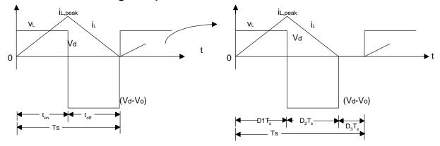
The volt-sec balance on the inductor  $\langle V_L \rangle_{Ts} = 0$  in DCM case to the right on the above figure gives:
