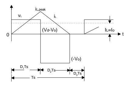
We can try to estimate  $D_2$  from the two equations that are true for all  $V_d$ (input) and  $V_0$ (output) cases.
