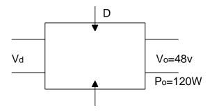
In steady state the output current in steady state is: (I\_o) =  $\frac{120W}{48}$  = 2.5 A
