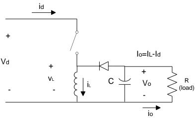
In the CCM of operation the  $V_{\rm L}$  and  $I_{\rm L}$  waveforms for buckboost are shown below.
