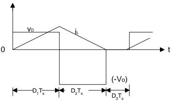
$\begin{array}{ll} \frac{V_{o}}{V_{d}} = \frac{D_{1}}{D_{2}} & \Rightarrow & \text{In a loss less converter operating in DCM} \\ & P_{o}(\text{out}) = P_{d}(\text{input}) \\ \frac{I_{o}}{I_{d}} = \frac{D_{2}}{D_{1}} & \Rightarrow \text{We can calculate the value at the border} \\ (I_{L})_{AV} = \frac{1}{2} (i_{L})_{peak} (D_{1} + D_{2}) \\ & \downarrow & \downarrow \\ \text{Height} & \text{time} \\ & = \frac{V_{d}}{2L} DT_{s} (D_{1} + D_{2}) \end{array}$
