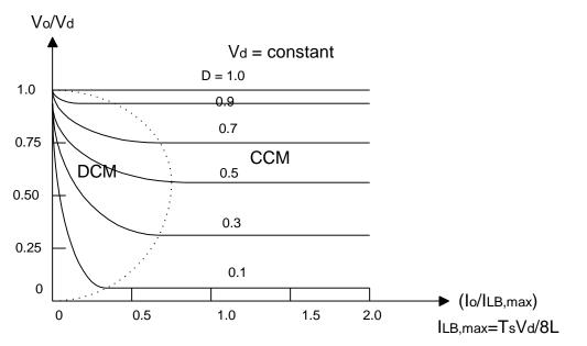
The DCM to CCM boundary depends on both D and  $I_{AV}/I_{max}$ . Note how V<sub>0</sub> /V<sub>d</sub> changes in DCM versus load current and is constant in CCM. We will revisit this in Chapter 10 of Erickson, especially Problem 10.3 which graduate students are to do for homework #2 now, undergraduates will do it later.
