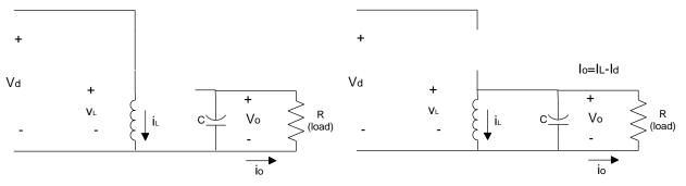
In steady-state the volt-sec on the inductor yields:  $\langle V_L \rangle_{Ts} = 0$ ;  $V_d DT_s + (-V_o)(1-D) T_s$ ;
