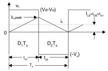
The effective DC inductor current is defined by the three equivalent parameters:  $I_{LB} = I_{OB} = I_{AV}$ . Where the subscript B refers to the boundary of CCM to DCM
