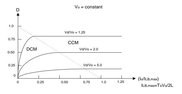
Similar plots of the DCM to CCM boundary can be made for the other two basic converter topologies as we will do below.
