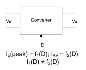
Whenever  $I_o(peak) > I_{AV}$  and unidirectional switches present $\Rightarrow$ DCM operation occurs with its mixed desirable and undesirable features both on a DC and AC basis.
