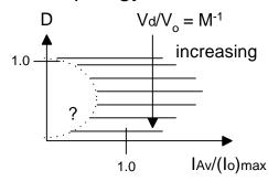
The above dashed line is CCM-DCM boundary transition for the <u>boost</u> topology in steay-state. To the left of the dashed line we will derive the non-ideal source characteristics, as compared to the ideal CCM voltage source curves.
