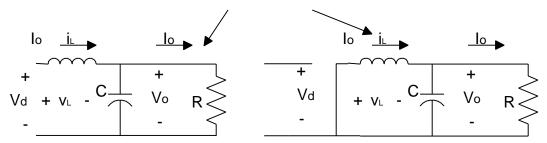
The above switch on and switch off circuit topologies are WRONG for the boost circuit. For HW#2 please draw the correct circuit topologies, that the equations below will satisfy by using the boost circuit below in two switch states.
