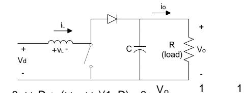
$$\langle V_L \rangle_{T_s} = 0; V_d D + (V_d - V_o)(1 - D) = 0; \frac{V_o}{V_d} = \frac{1}{1 - D} = \frac{1}{D'}$$
