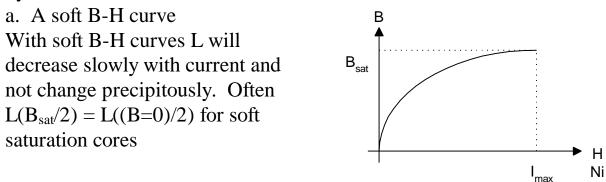
However above  $B_{sat} \ \mu \to \mu_o$  and  $L \to short circuit or very small values$  $Then for B>B<sub>SAT</sub> we find <math>L = \frac{m_o A_c N^2}{\ell_c}$  where we replace  $\mu(core)$  by
