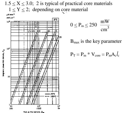
Most PWM converter  $i_L$  waveforms are square or triangle waves not sinusoids. These signals contain DC components. B(dc) causes no core losses only core saturation! Harmonics of the switch frequency also occur for many converter waveforms  $\Rightarrow$  Higher core losses due to the f<sup>2</sup> dependence of eddy current losses.
