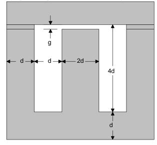
I<sub>DC</sub> >> I<sub>ac</sub> Case for Filter Inductors
