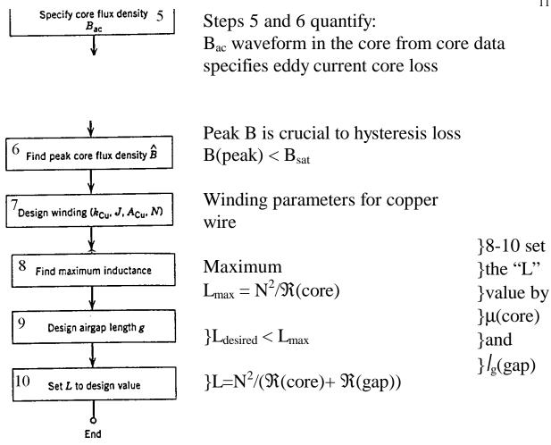
b. Detailed Approach for Each of 10 Steps For HW#1 verify the specific quantities in the example below on the left hand side.
