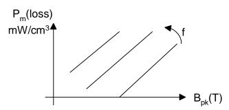
From  $P_M$  vs  $B_{pk}$  vs f or from the chosen core data base we find B and then  $P_m$ . Where  $P_m$  is Specific Power density. Take as illustrative for 3F3 core under the above conditions  $\approx 250 \text{ mW/cm}^3$ .
