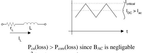
$I_L^2$  (rms)<sub>rL</sub> > core loss
