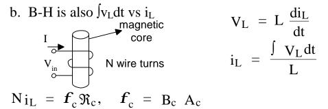
For  $V_{in}$  to the inductor being a sinusoid or any waveform the  $\phi$  increases to a peak only after integrating  $V_L$ . A step of  $V_L$  is easiest to visualize.
