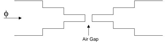
Both core and wire winding losses as well as saturation effects establish design rules for those who "wind their own inductors" as shown below. Limitations of magnetic cores are crucial to good inductor design
