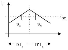
In many cases the di/dt upward slope  $(s_u) \neq$  downward slope  $(s_d)$  in a/sec units. this means that we must choose d and d' so that the integral is indeed zero. That is volt-second balance sets d values to their proper values in steady state.
