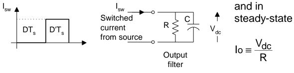
FOR A SPECIFIED  $\Delta v$  RIPPLE GOAL, THE VALUE OF C DEPENDS ON  $f_{sw},$  D,  $V_{DC},$  R
