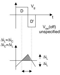
Assuming  $v_o$  varies little, this is the voltage waveform across the inductor  $v_L$  for:  $v_{sw}(on)$  (DT<sub>s</sub> circuit):  $V_L=V_g-V_o$  $v_{sw}(off)$  (D'T<sub>s</sub> circuit):  $V_L$  unspecified This voltage variation across  $V_L$  causes a  $\Delta i_L$  flowing through L about I<sub>DC</sub> Shaded area under the  $\Delta i_L$  vs t curve shown is positive Q<sub>C</sub> during T<sub>s</sub>/2. This will cause a  $\Delta v_C$ .
