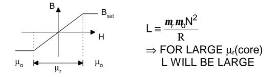
If **b** in inductor core exceeds  $B_{sat}$  the L value will decrease by 10-10<sup>3</sup> at B >  $B_{sat}$ . This means L(i) variation occurs in a threshold fashion, not gradually. Finally, for steady-state to occur over the full cycle of the switch waveform t<sub>s</sub> THE NET  $\int_0^{T_s} v_L dt \equiv 0$ . THIS MUST OCCUR, OTHERWISE THE INDUCTOR CURRENT WILL GROW EACH CYCLE AND EVENTUALLY REACH SATURATION AND i > i(critical).
