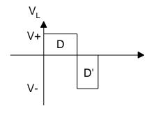
For an inductor in steadystate and well below core saturation, the total integral area v<sub>L</sub>dt over T<sub>s</sub> is ZERO.
