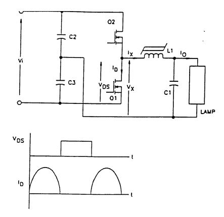
$$V_{\chi}(\omega t) = \frac{2\sqrt{2}}{\pi} V_{IDC} \sin(\omega t)$$
