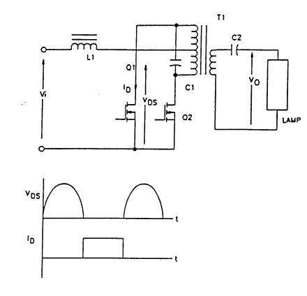
$$V_{OC}(\omega t) = \frac{\pi}{2\sqrt{2}} V_{IDC} \sin(\omega t)$$
