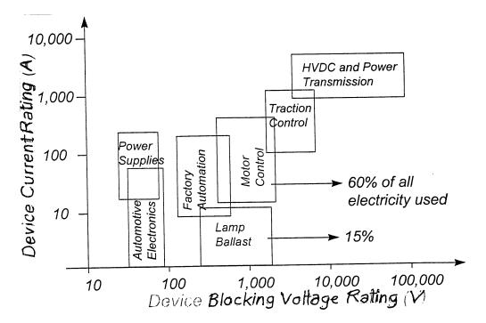
Clearly, we have different applications that place specific requirements on the solid state switches. Only as advances in solid state switches occurred could these new applications become cost effective. Switch technology is an enabling one for new applications. Two issues are enabling: electrical peformance and cost.
