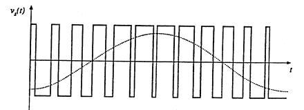
The switch fequency is  $f_{sw}$  and is chosen so that  $f_{sw} >> f_{out}$ .  $f_{out}$  is chosen by duty cycle of on-off of the switch. Typical pulse-width-modulated switch voltage and its low frequency component. V sin  $\omega_{out}$ t, V =  $f_1(D)$ ,  $\omega_{out} = f_2(D)$ This course provides details on how we achieve this.
