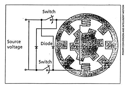
[3] The switched reluctance motor is diagrammed as a simplified eightpole stator and a six-pole rotor machine. Torque is developed by the tendency of a magnetic circuit to adopt a configuration of minimum reluctance (to maximize the magnetic flux). This tendency translates into a rotation of the rotor so that its poles align with the stator's poles. These pole pairs are in turn energized sequentially from a dc source through electronic switches, thereby creating the rotating torque.
